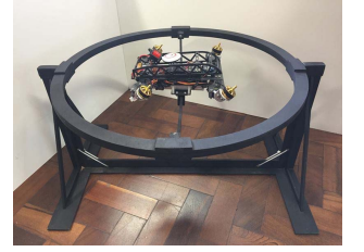
(b) Illustrative picture of the gyroscopic test bench system after its assembly with a quadrotor UAV.
